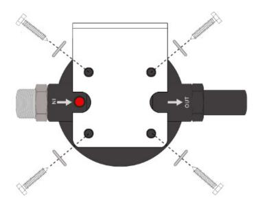
Locate Box #2. Using four (4) of the lag bolts and washers from this box, attach the mounting bracket to the post-filter cartridge filter housing cap as shown in the diagram below. Note that this time, the fittings will be reversed. The black plastic stem fitting should be on the left (inlet) the stainless steel threaded fitting should be on the right (outlet).
