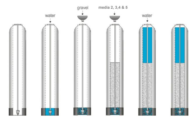
Once you have finished adding the media to the tank, remove the tape from the distributor tube. Be careful not to pull upwards on the riser tube while doing this as it is important that the distributor remain in its recess at the bottom of the tank.
